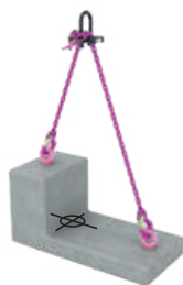
Asymmetrical load Centre of gravity off-centre
