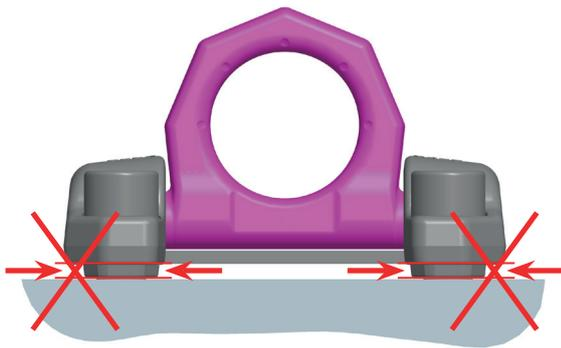
Pic. 1: The lifting point must have been fully bolted in.
